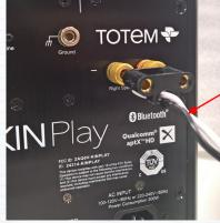
Once the plugs have been removed, connect the two speakers together with the supplied speaker wire.
